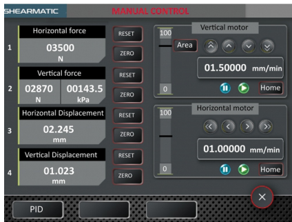
Screenshot of the manual control mode of the horizontal and vertical stepper motors. Transducers readings, vertical yoke position and horizontal force are shown in real time
